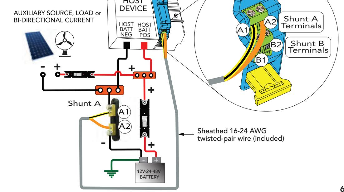
**Figure 2 - Auxiliary Current Application**
