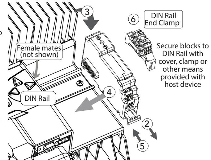
**CONFIGURATION** - first connect the battery to the host device to power host device-shunt block system
