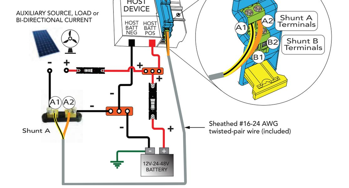
**Figure 3 - Net Battery & Auxiliary Current Application**
