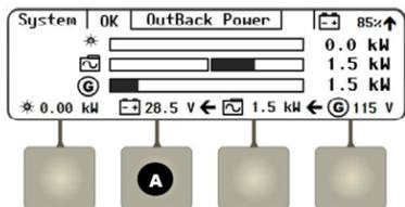
If the FLEXnet DC (FN-DC) battery monitor is installed, the **<Battery>** soft key (A) opens screen A1.
