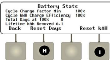
From the **Battery Status** screen, the **<Stats>** soft key (E) opens the **Battery Stats** screen. This shows long-term battery statistics.
