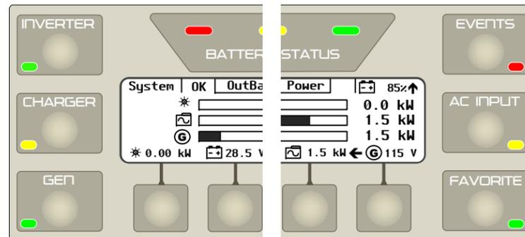
**EVENTS** indicator (red): An “event” is a change in status, externally imposed on a device on the HUB (an on/off command, an automatic generator start, loss of grid power, etc.). The **Event History** screen logs all events for potential troubleshooting (see page 17). The LED indicator means that an event requires acknowledgement. Usually it only illuminates when a fault occurs.
