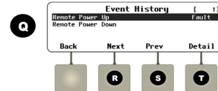
The **EVENTS** hot key (Q) brings up **Event History**. (See page 5 for the definition of an event.) This screen can scroll through each event and display the details to determine if corrective action is required. An event may need acknowledgement before the **EVENTS** LED indicator will turn off.
