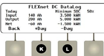
From the **Battery Status** screen, the **<DataLog>** soft key (G) opens the **FLEXnet DC DataLog** screen. It maintains a continuous daily log (up to 400 days) of amp-hour, watt-hour, and SOC statistics. One day can be displayed at a time.
