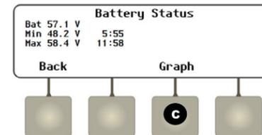
The **<Graph>** soft key (C) brings up a single graph showing changes in battery voltage over time. This graph may be used by other soft keys.
