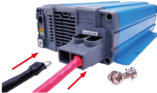
Figure 17. DC cable connection
