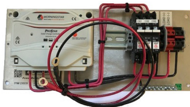
PRE Control Panel with a 30 amp ProStar
