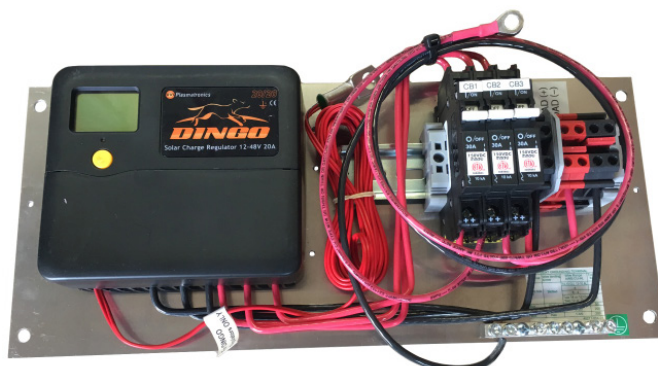
PRE Control Panel with a 20 amp DINGO
