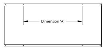
MEASURE DIMENSION (A) ON THE SOLAR PANEL TO DETERMINE WHETHER THIS SMALL SP BUCKET MOUNT WILL WORK IN AN OVER THE TOP OF POLE CONFIGURATION..
