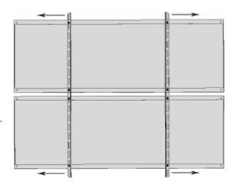
D. Secure the rails with a  $1/4-20 \times 3/4$ " bolt, lock washer, and hex nut in each of the PV mounting holes (4 on each panel). Tighten the bolts to 84 in-lbs.
