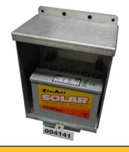
The SunWize Power & Battery E1-38 is a versatile mill-finish enclosure that can serve as a small self-contained battery box, a combiner box, or many other purposes. Three bottom 1/2" knockouts, two rear 1/2" knockouts, and two side 1/2" knockouts.
