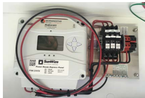
Pre-wired 230058 Control Panel with PS-40M-MPPT
