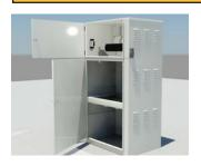
UPS style enclosure targeted for battery backup system applications. NEMA3R rated, white powder-coated aluminum enclosures feature hinged, key lockable doors with dust covers on locks and gasketed door. Passive cooling ventilation. Three 1-½" electrical knockouts per side. Significant space for controls allows up to (16) customer load breakers, plus multiple battery chargers and/or controllers. Power Ready Express (PRE) Control Panels do not fit in UPS style enclosure.
