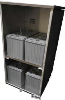
The SunWize Power & Battery C4-500 alumiunum enclosure features a mill-finish and a NEMA3R rating for indoor or outdoor use. The C4-500 enclosure can mount on a flat vertical surface or on a variety of pole sizes. It also features pad-lockable lift off doors and passive cooling ventilation.
