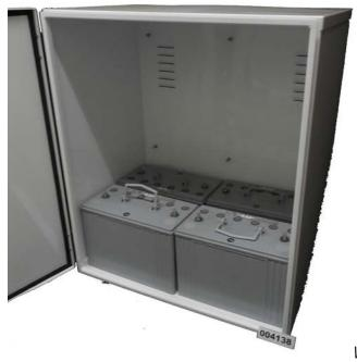
The SunWize Power & Battery WF4 alumiunum enclosure features a white powder-coated finish and a NEMA3R rating for indoor or outdoor use. The WF4 enclosure can mount on a flat vertical surface or on a variety of pole sizes. It also features hinged, key-lockable doors with dust covers on locks and gasketed door. Passive cooling ventilation. Two rear ½" electrical knockouts and two rear 1" electrical knockouts.
