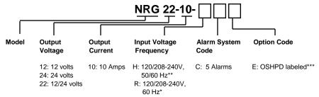
NOTE: Not all configurations are available on all models. Contact the factory for confirmation. All NRG models are C-UL Listed to UL 1236.
