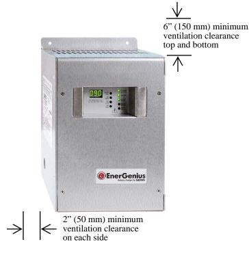
Mount to vertical surface of 3/4" (19 mm) plywood or other material of equal strength and durability, using four mounting screws 1/4" (6 mm) diameter.
