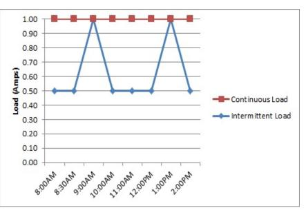
at different times of the day. Typical non-continuous loads are lighting, radios on transmit, valves or actuators, pumps or motors, gate openers, etc.
