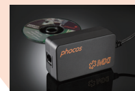
MXI Interface for MCU communications with computer RS232/USB interface
