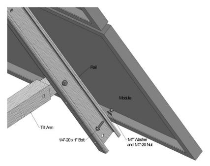
9. Securely fasten entire structure and use ballast as needed.
