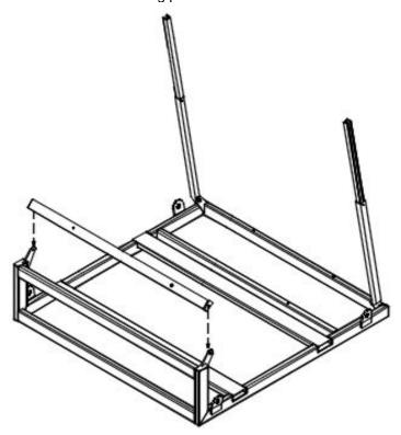
4. Attach a second cross bar to the free ends of the tilt legs using provided 3/8" hardware.
