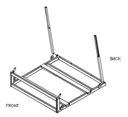
3. Attach one cross bar to front tabs using provided 3/8" hardware.
