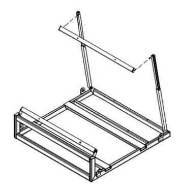
5. Attach module rails to both front and back crossbars using provided 5/16" hardware. Mount module rails to cross bar based on which holes align with desired solar module.
