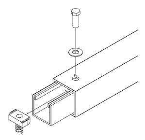
2. Attach tilt legs to the rear steel base tabs using the provided 3/8" hardware.
