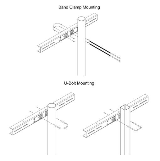
3. Loosely fasten the lower saddle to the pole. Use the below chart for rough spacing between the two saddles.
