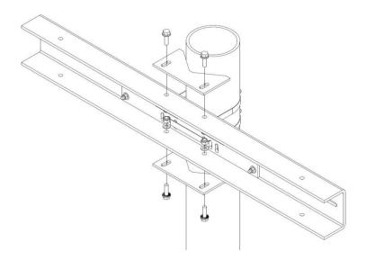
9. Check alignment of all assembled parts and ensure all bolted connections are tight.
