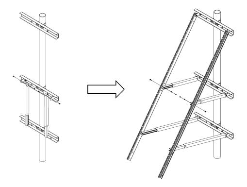
8. Attach a bearing plate to the top and bottom of each saddle bracket with the provided 3/8" hardware. Push the plates tightly against the pole and tighten the bolts. <u>Optional</u>: For 12"-24" poles, use the bearing plates provided in the large pole adapter kit. **USE ANTI-SEIZE**
