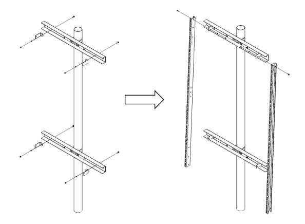
6. Attach tilt legs to lower saddle L-brackets. Adjust the tilt angle by adjusting the tilt arms and lower saddle to the desired angle of tilt then tighten the U-bolt/band clamp on the lower saddle. For 5/16" hardware tighten using 1/2" wrench to 10-12 ft. lbs. torque, for 3/8" hardware, tighten using 9/16" wrench to 18-20 ft. lbs. torque. USE ANTI-SEIZE
