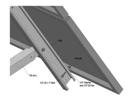
10. Mount the solar modules to the rails using the 1/4" hardware provided. USE ANTI-SEIZE
