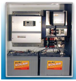
The SunWize Power & Battery WF2 alumiunum enclosure features a white powder-coated finish and a NEMA3R rating for indoor or outdoor use. The WF2 enclosure can mount on a flat vertical surface or on a variety of pole sizes. It also features feature hinged, key-lockable doors with dust covers on locks and gasketed door. Passive cooling ventilation. Two rear ½" electrical knockouts.
