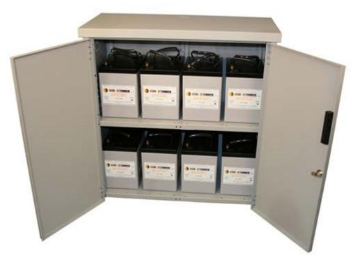
Battery Enclosure with locking door and one shelf. Holds eight group 31 or sealed golf cart sized batteries. Gray powder coated steel. Two cabinets can be stacked horizontal or vertical for expansion. Ships knocked down in two cartons. Battery are not included.
