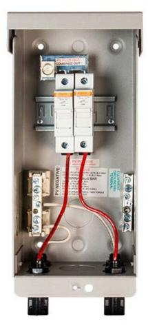
The Pre-wired MNPV2 combiner is rated for outdoor use. Designed for combining high voltage strings using 10mm x 38mm fuses up to 60A total. The use of touch safe din rail mount fuse holders and fuses allow operation up to 600 Volts. The MNPV2 is rated for up to 60 amps.
