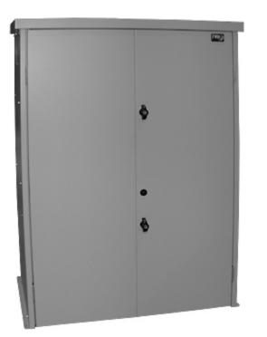
Battery Enclosure with locking door. Holds eight L16 batteries on two shelves. Holds 12 group 31 or golf cart batteries with additional shelf. Gray powder coated steel. Two cabinets can be stacked horizontal for expansion. Use the "Large back up kits" to have 2 shelves of batteries plus inverter & charge controller on the top 3rd shelf. Ships knocked down in two cartons.
