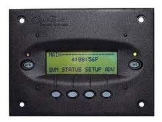
The **Mate2** is a complete Outback system control module and display for inverters and FlexMax controllers in any combination. Its display shows operation and allows programming and adjustment of inverter and controller set points. It can be located up to 1,000 feet away from the system and includes an RS232 port for connection to a PC for data logging and system monitoring.
