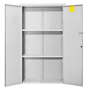
MNBE-C Battery Enclosure with locking door and three shelves. Holds twelve group 31 or sealed golf cart sized batteries and even the 14" tall PVX-3050T from Concorde. MNBE-C battery enclosure accepts MNEDC175 or 250 breakers. Gray powder coated steel. Two cabinets can be stacked horizontal for expansion. Enclosure size: 36.5" wide x 16" deep x 55" tall/261 Lbs including pallet (freight truck only)
