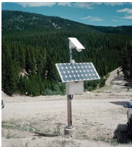
A SunWize® Power Ready System provides power to a water reservoir monitor in the Colorado mountains.
