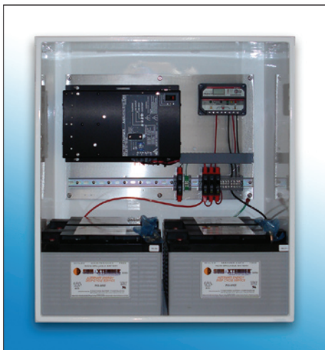
600 watt Power Online System with 48Vdc, 120AH VRLA batteries, and custom system options
